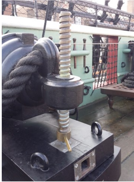
Figure 6 – Screw Elevating Mechanism Fitted to a Carronade
