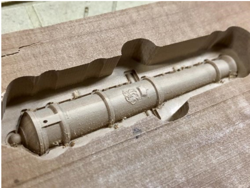
Cannon made with 2-sided CNC machining
