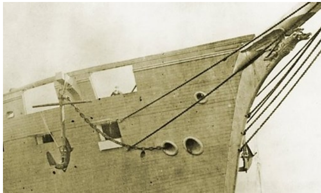
Figure 6 – Dual Pivot Gunport Arrangement Crop of a photograph (public Domain) of the Russian Frigate General Admiral , 1858.
