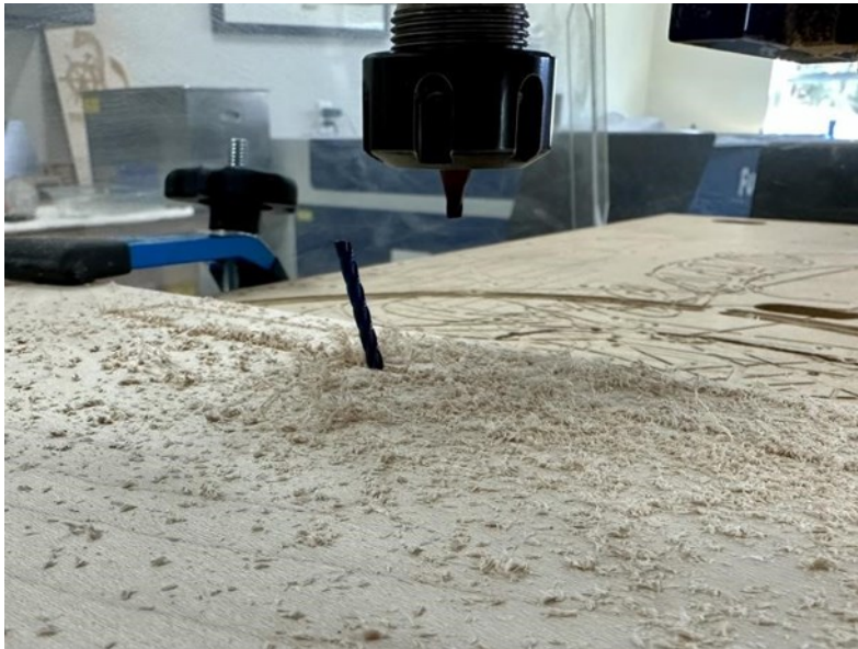
Broken endmill caused by tool path error
