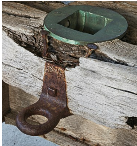
Figure 15 – Train Tackle Eye Plate fitted to the Warrnambool Casemate Gun Author's Photograph (©2016)
