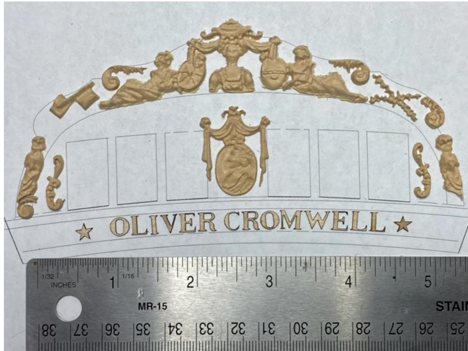
Then we create a CNC toolpath to carve scale replicas of the parts in boxwood
