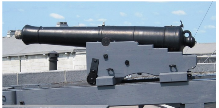
Figure 9 – Blomefield Pattern Gun with Dispart and Millar Sight From Harold A. Skaarup's Silverhawk Website – Photograph by Doug Knight
