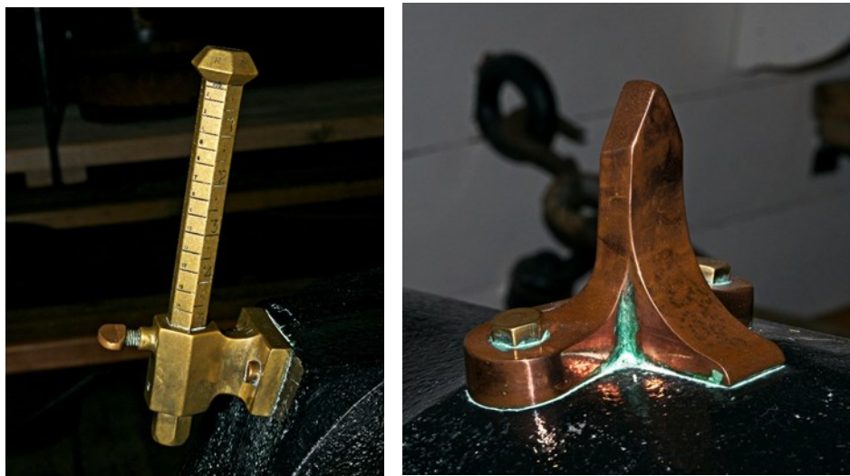
Figure 8 – Millar (L) and Dispart Sights (R) fitted to HMS Warrior's Broadside Guns Author's Photographs (©2020).
