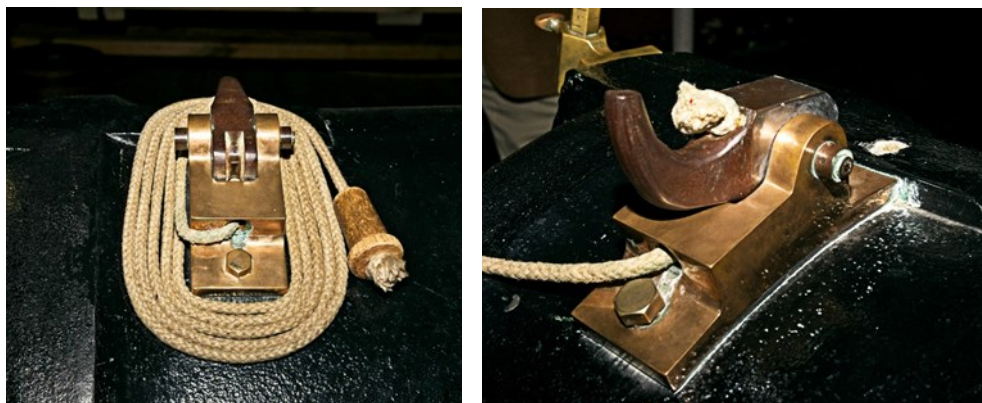
Figure 4 – A Dundas Style Gunlock fitted to HMS Warrior's Broadside Guns Author's Photographs (©2020)
