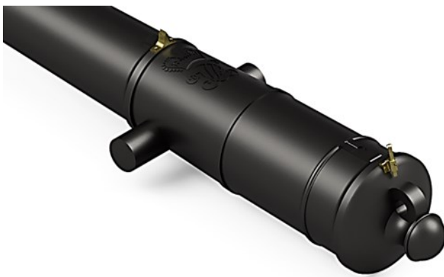
Figure 10 – Sights as fitted to the Blomefield Gun in HMCSS Victoria Render illustrated by, and used with permission of, Chris. Ramsay ©2022
