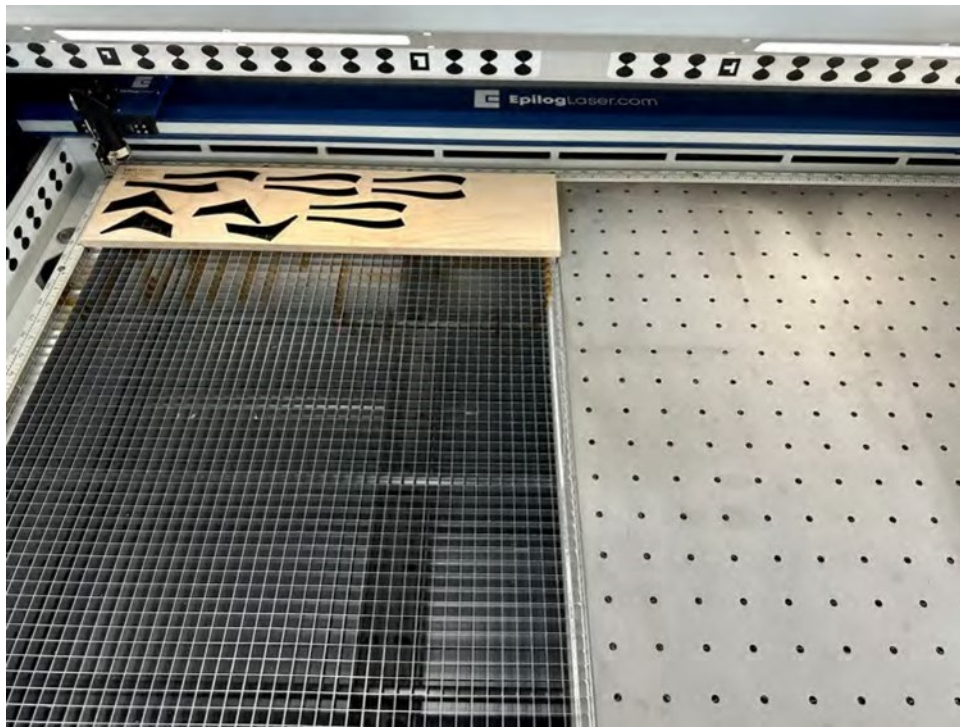
Mesh/grid bed for cutting on the left, vacuum table bed for engraving on the right
