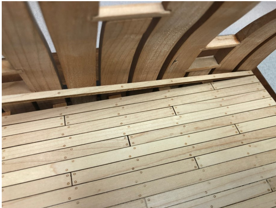
Laser cut planking with char edges to simulate caulk and engraved treenails
