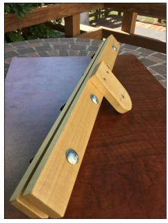
When assembled, cut the 1" X 1" X 1" "saddle in place on part G. Glue the two knuckle parts together as shown. When dry, add reinforcing screws to the knuckle where appropriate.
