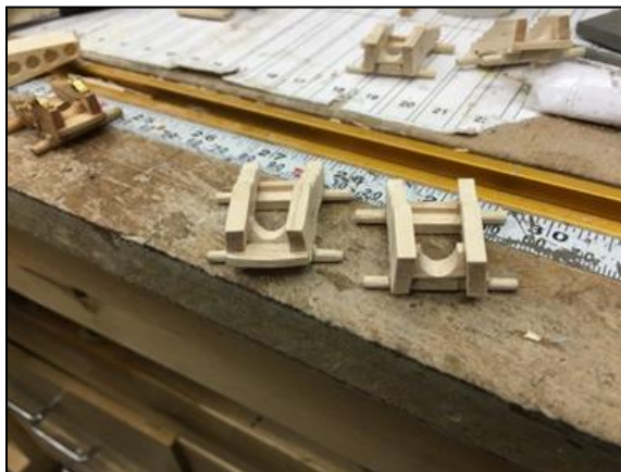
The carriage on the left has had the transom ledge installed
