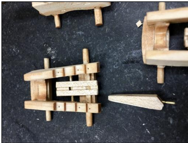
Carriage with Quoin bed in place. The quoin is to the right. Notice also the holes drilled in the steps of the carriage. Pins will be glued in place to mimic the bolts through the assembly.
