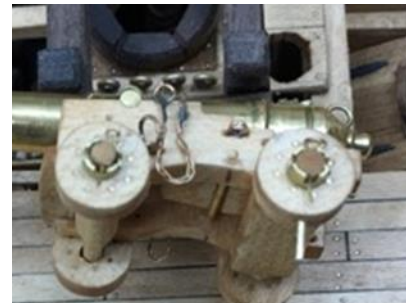
Long Gun showing stern truck pins and capsquare chain installed.
