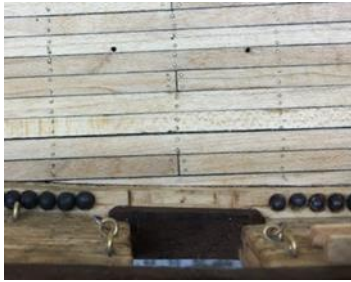
Holes drilled for a long gun.
