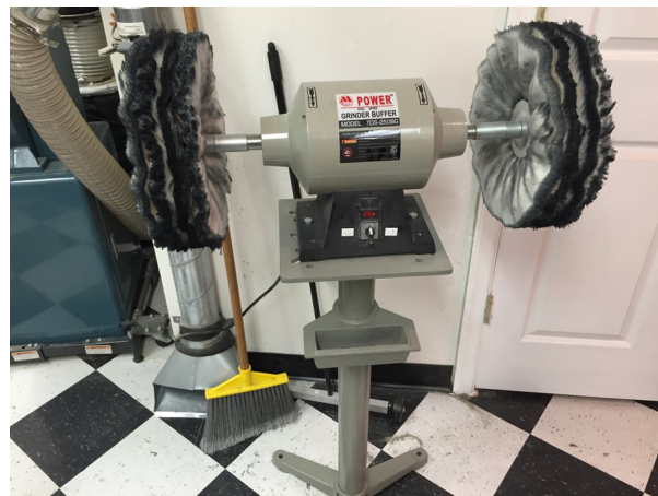
Figure 13 - The power buffer
