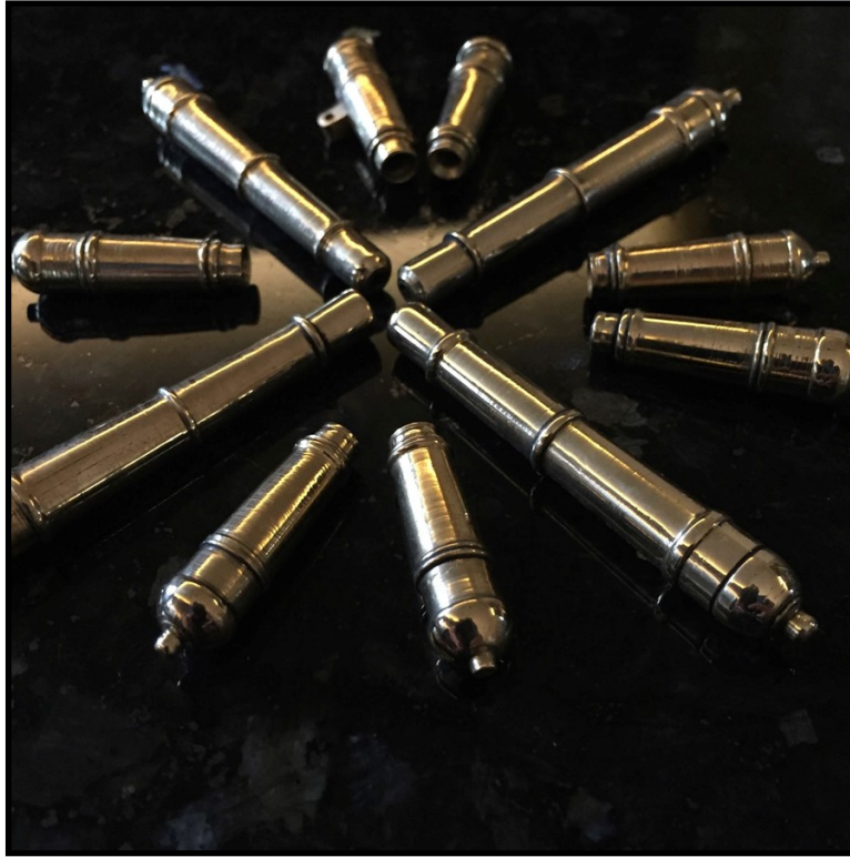
Figure 14 - Final turned barrels. Note the upper left Carronade has already been fitted with the pivot point. This will be covered in a future article
