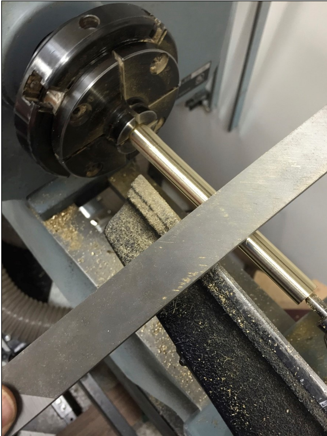
Figure 8 - The long angle file was used in the final truing. Notice the clogged teeth on the upper edge of the file. These must be cleaned before using this side again or it will result in scoring of the finish
