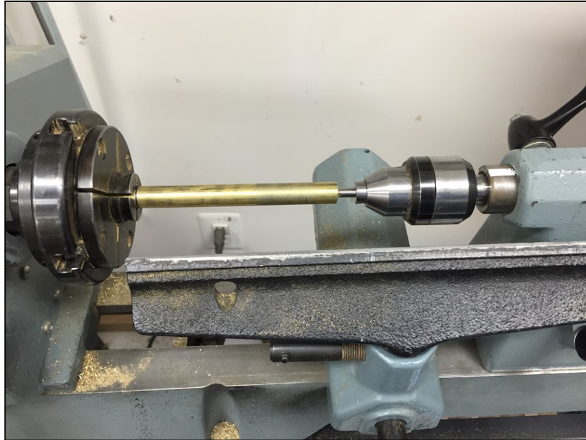
Figure 6 - Once the barrel is bored the live center is moved into the bore to stabilize the rod for truing
