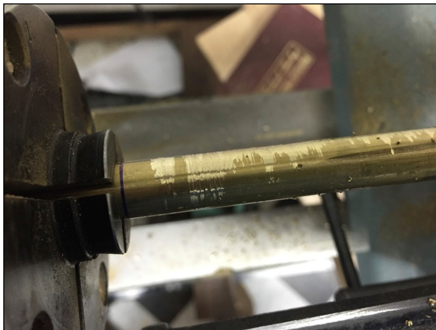
Figure 7 - The rod after starting the truing. The shiny areas are where material has already been removed. Once trued, the rod will not have any dull areas along its length
