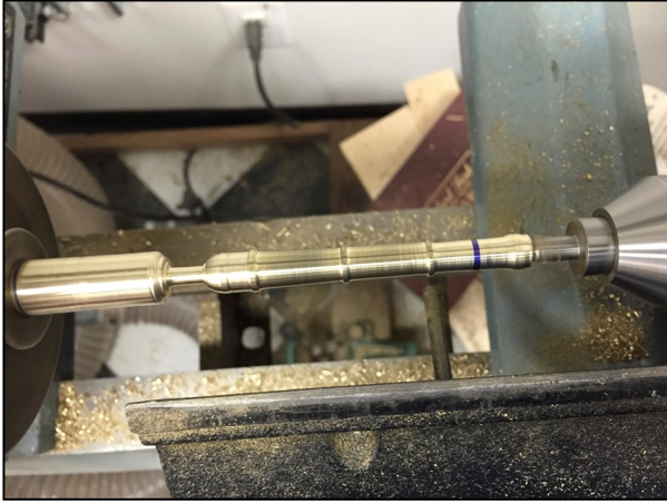
Figure 11 - Once the barrel has been shaped, I re-marked the muzzle end for parting
