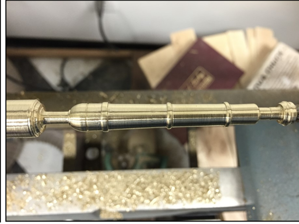
Figure 12 - The muzzle end cut down. Since it is already bored, this is nearly parted at this point
