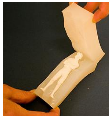
Photo 10. Urethane figure in its silicone mold.
