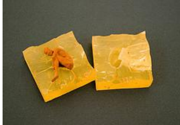
Photo 7. Silicone mold with seated clay and wax figure.
