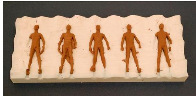
Photo 8. Silicone gang mold with clay and wax figures.
