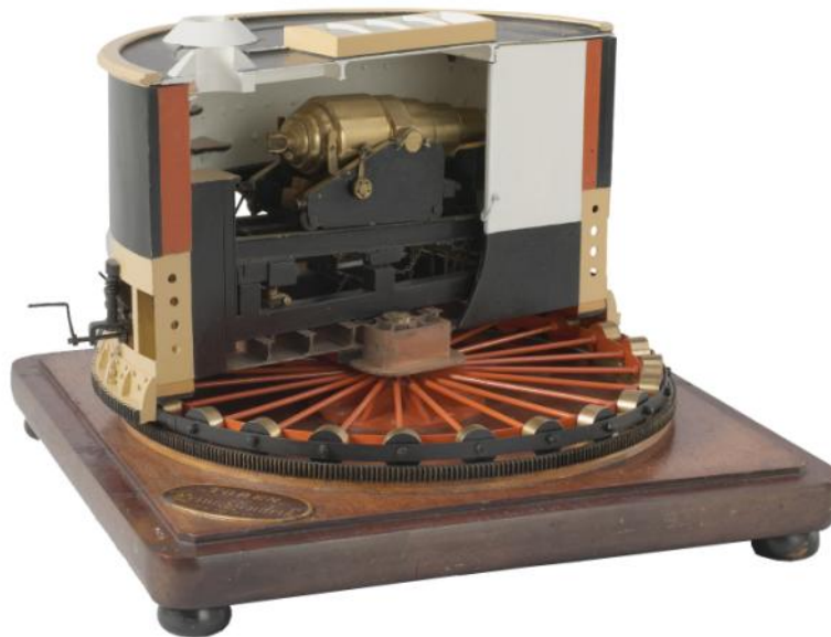
Model of a cross-section of an armoured gun turret, 1868 (NG-MC-1244)
