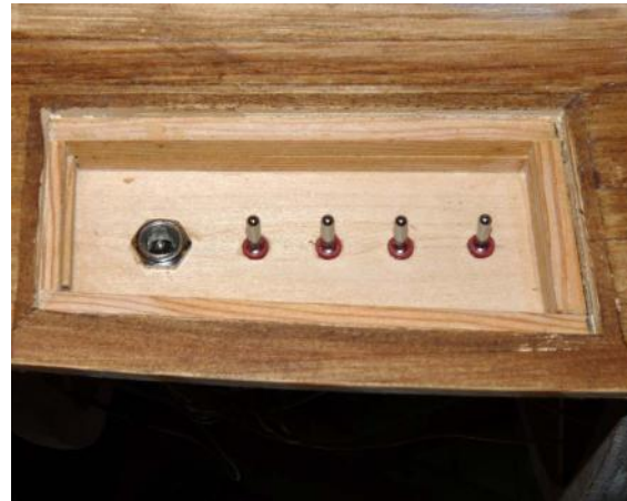
The switches themselves will be accessed via the port side cover that on the full size boat gives access to the petrol tanks.
