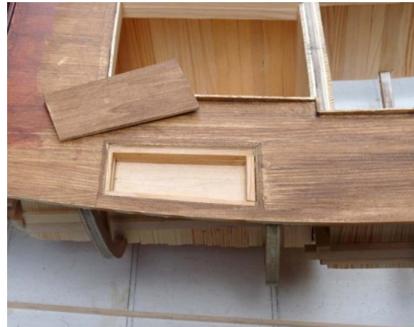
The inspection hatch on the port side of the deck has been made removable to allow for the fitting of the switches that will control the motors, lights etc.
