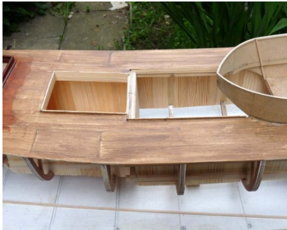
The internal walls of the engine room and the survivors cabin have been planked along with the deck.
