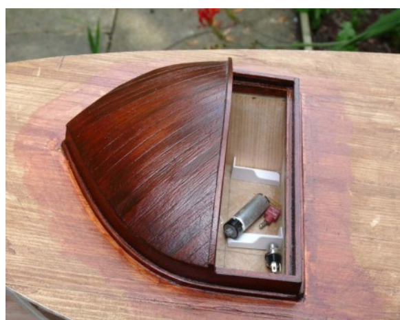
The forward cockpit has also been built up and the turtleback over it planked and varnished.
