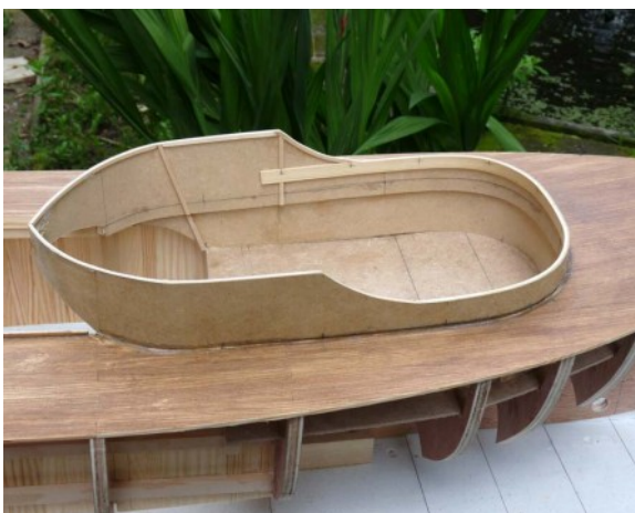
The walls of the rear cockpit have been built and are ready for the addition of the external planking.
