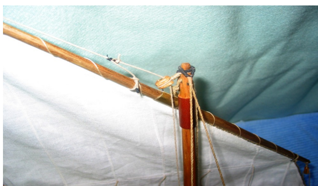
Mast head showing stays, uphaul (through mast) and topping lift
