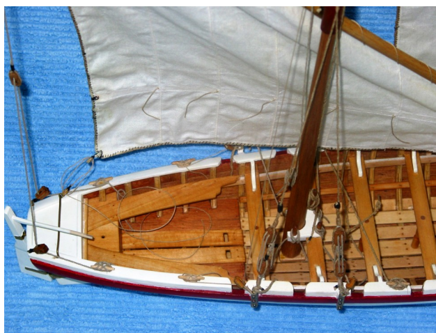
Stern view showing lockers and masting step
