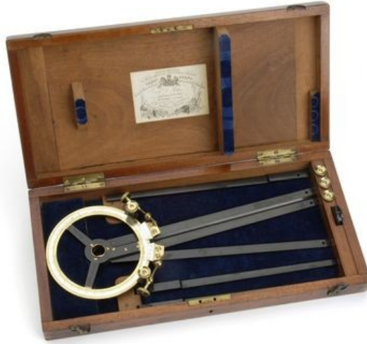
Station Pointer Circa 1850 made by John Dennett Potter of London England
