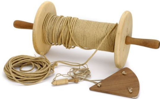
Log Reel, Line and Log-ship
