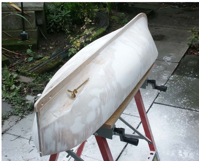
With the first layer of planking completed the hull is sanded and faired.
