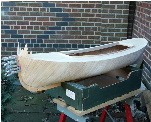
With the first layer of planking completed the hull is sanded and faired.
