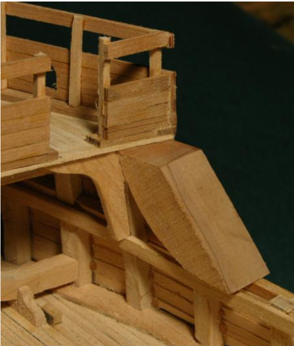
A slightly oversize thickness of the cap rail is drawn on the side of the block and cut out.
