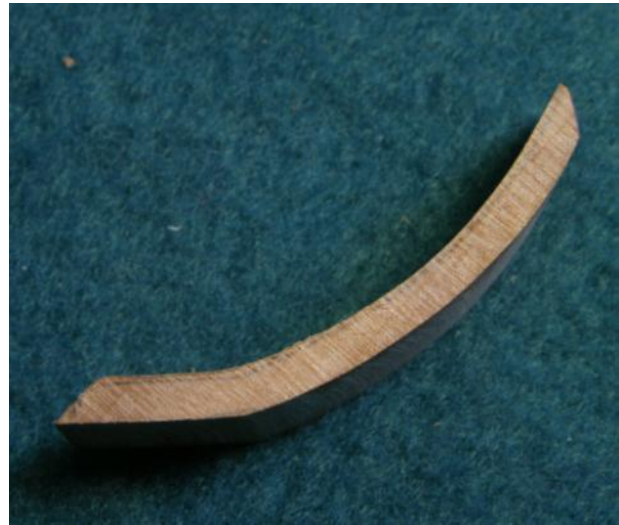
A slightly oversize thickness of the cap rail is drawn on the side of the block and cut out.
