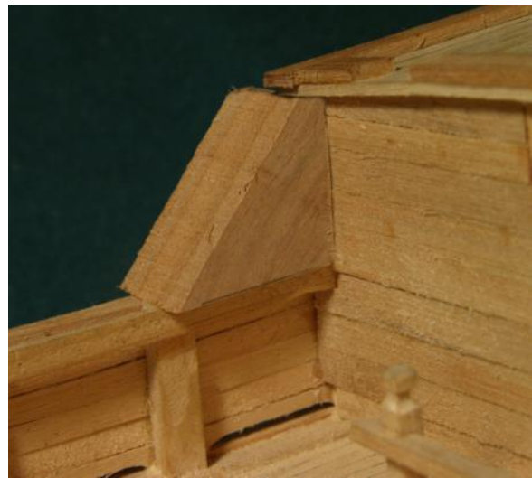
A slightly oversize thickness of the cap rail is drawn on the side of the block and cut out.
