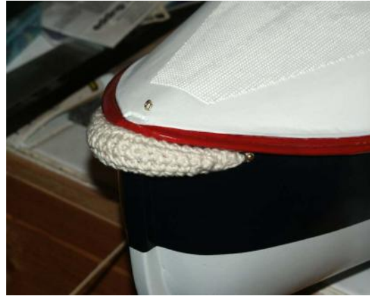
The bow bumper was crocheted by my wife and when fitted gives the boat its typical RNLI 'look'.
