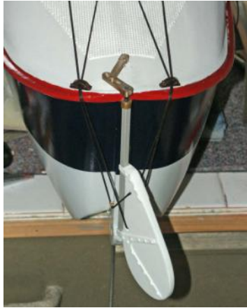
The lifting rudder has been fitted along with the appropriate lift lines.
