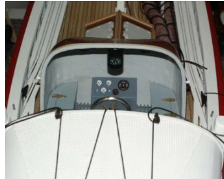
All the engine controls have been fitted inside the mechanics shelter and the working compass hung where the helmsman can easily see it.
