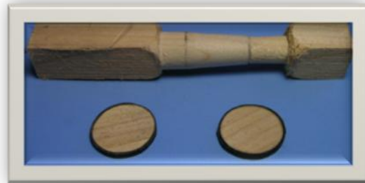
Building the rest of the capstan began with turning the spindle to the measurements
