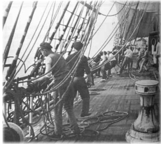
Pulling up the Port Main Brace
