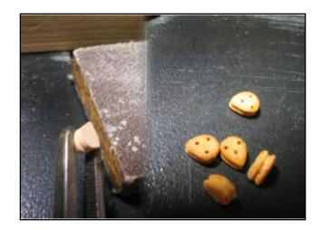
Finally drill three holes and paint ready dead eyes. It took around an hour to produce 10 such deadeyes.
