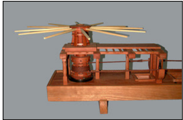
View of the double headed capstan showing drumhead and trundlehead with messenger in place.
