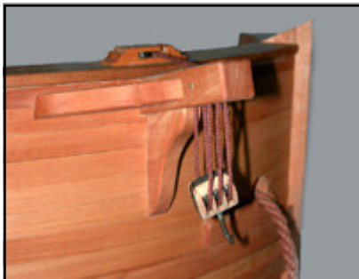
A strong piece of timber called a cathead projected from the bow. Ironbound cat blocks were used to catch the anchor ring and hold the anchor clear of the hull while being raised and lowered. Sheaves were fitted into the cathead for the lifting tackle.
