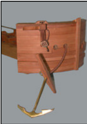
Bow of the ship, showing the cathead, hawse holes and anchor.
