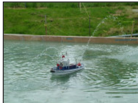
This model of the Hamilton Fire Tug "Judge McComb" had it's first launch since being build by their master builder Don Hodgson. This is built on a scale of 1 inch to the foot with 3 pumps for the fire nozzles. All of Don's boats are scratch built..
